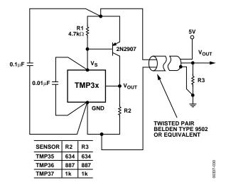
Figure 32. Remote, 2-Wire Boosted Output Current Temperature Sensor
