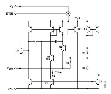
Figure 22. Temperature Sensor Simplified Equivalent Circuit
