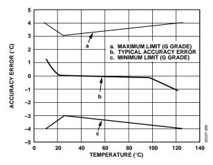
Figure 7. Accuracy Error vs. Temperature
