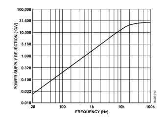
Figure 9. Power Supply Rejection vs. Frequency
