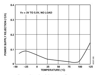
Figure 8. Power Supply Rejection vs. Temperature
