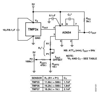
Figure 34. Temperature-to-Frequency Converter
