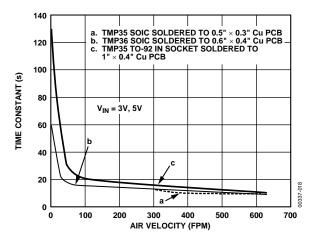
Figure 18. Thermal Response Time Constant in Forced Air
