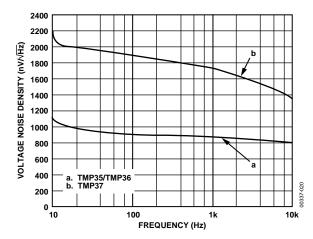
Figure 21. Voltage Noise Spectral Density vs. Frequency
