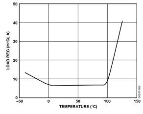
Figure 5. Load Regulation vs. Temperature (m°C/ $\mu$ A)
