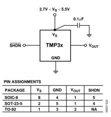
Figure 24. Basic Temperature Sensor Circuit Configuration
