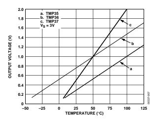
Figure 6. Output Voltage vs. Temperature
