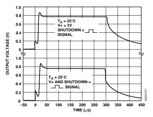
Figure 16. V<sub>OUT</sub> Response Time to Shutdown and V+ Pins vs. Time
