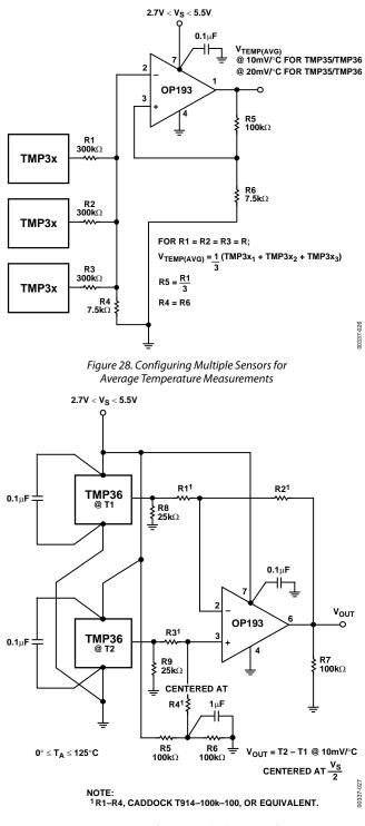
Figure 29. Configuring Multiple Sensors for Differential Temperature Measurements
