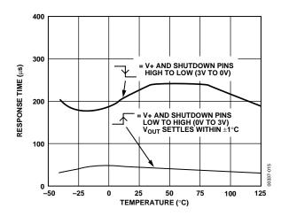
Figure 14. Vout Response Time for V+ Power-Up/Power-Down vs. Temperature
