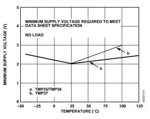
Figure 10. Minimum Supply Voltage vs. Temperature
