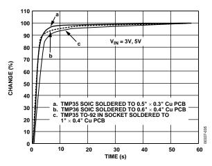
Figure 19. Thermal Response Time in Stirred Oil Bath
