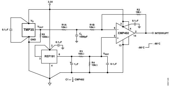
Figure 30. Pentium Overtemperature Interrupt Generator
