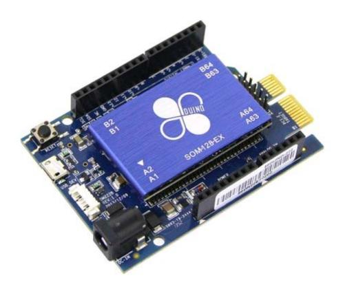
86Duino is an open-source embedded platform based on Vortex86EX SoC, easy-to-use hardware and software integrated. This Arduino-compatible board can support many x86 O/S as well as those running on the original Arduino base system.
