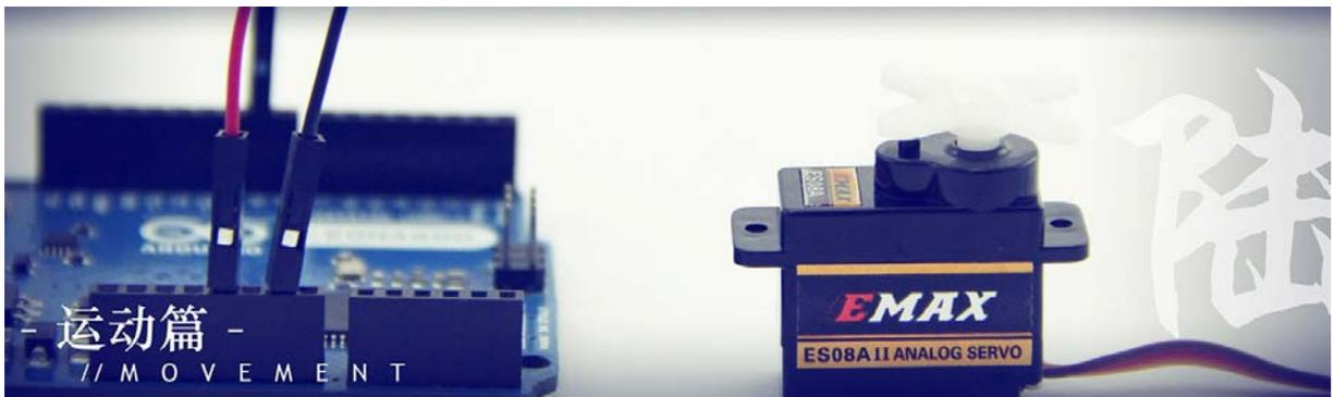
Servo motor (servo) is commonly used in small robots and other machines to control angular position. It is wrapped by a small gear box, and positioned by the timing control pulses. In this section we control the angular position of the mini servo with the help of potentiometer.
