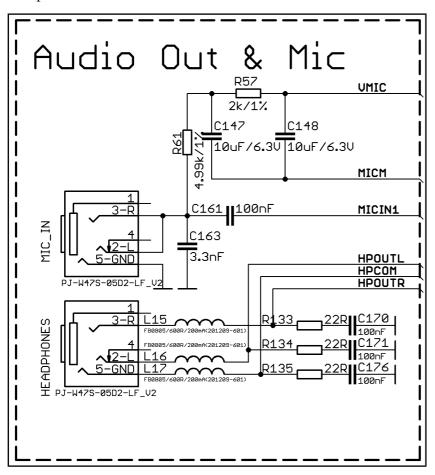
Standard MIC\_IN jack is mounted for audio input to the board. Note that it is a single channel MIC\_IN. The MIC\_IN is a mono input.
