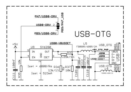
The USB\_OTG features Low Loss Power Distribution Switch SY6280 which protects the board in case the devices you have plugged to the USB\_OTG attempt to draw more current than 523mA combined. The maximum current available on the 5V USB\_OTG is exactly 523mA.
