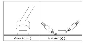
Avoid rubbing or scraping the resin by any object, during high temperature, for example reflow solder etc.
