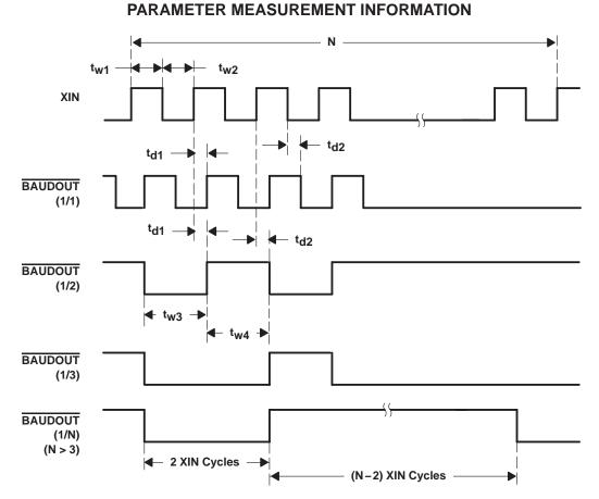
Figure 5. Baud Generator Timing Waveforms
