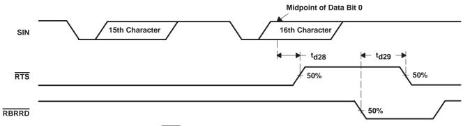
Figure 19. Auto-RTS Timing for RCV Threshold of 14 Waveforms
