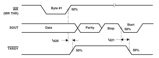
Figure 14. Transmitter Ready (TXRDY) Waveforms, FCR0 = 0 or FCR0 = 1 and FCR3 = 0 (Mode 0)
