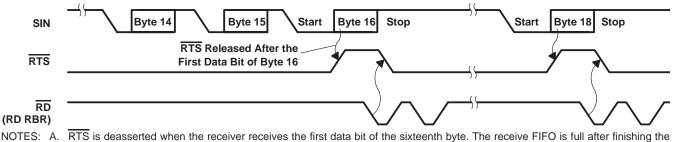
NOTES: A. RTS is deasserted when the receiver receives the first data bit of the sixteenth byte. The receive FIFO is full after finishing the sixteenth byte.
