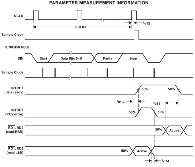
Figure 8. Receiver Timing Waveforms
