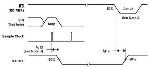
NOTE A: This is the reading of the last byte in the FIFO.
