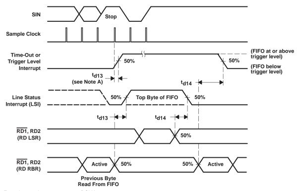
NOTE A: For a time-out interrupt, t<sub>d13</sub> = 9 RCLKs.
