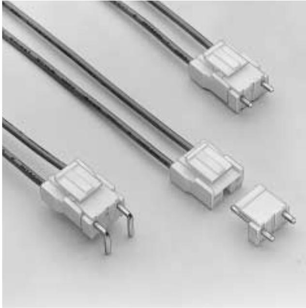
**This 7.92mm (.312") pitch large current carrying capacity connector is used with primary power supply circuits and various other circuits requiring large currents. It features an anti-misinsertion construction and a reliable locking mechanism to ensure maximum safety.**
