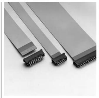
The FMZ series, a Zero Insertion Force (ZIF) connector series, was developed to increase wear resistance and extend the connector's mating life. It is a very compact connector with a thickness of only 4.2mm (.165") and a pitch of only 1.0mm (.039") and is thus useful for high density packaging. The contact has a reliable double-leaf construction which provides stable connection.
