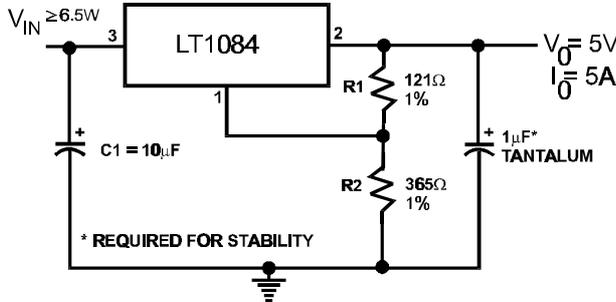
$$V_{out} = V_{REF} \left( 1 + \frac{R_2}{R_1} \right) + I_{ADJ} R_2$$
