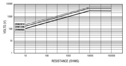
Test Method: 1.2/50 µs Waveform with 12 Ohm Resistor, 5 Pulses at 12 Second Intervals
