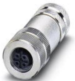
Bus system connector, PROFIBUS, INTERBUS, 5-position, shielded, Socket straight M12, B-coded, Screw connection, Knurl material: Zinc die-cast, nickel-plated, External cable diameter 6.5 mm ... 8.5 mm
