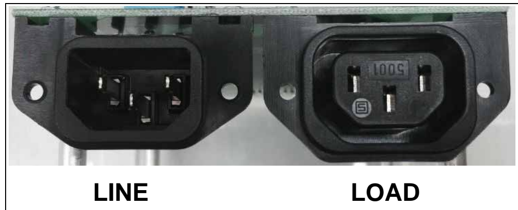
FIGURE 2-1: Connecting the MCP39F511A Power Monitor Demonstration Board.
