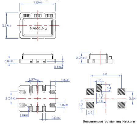
Contact Pads are gold over nickel Figure 2, Package drawing
