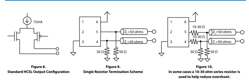
The VC-709 incorporates a standard High Speed Current Logic, HCSL, output scheme which is a 15mA current source switched between Out and Complementary Out. Being un-terminated drains, as shown in Figure 8, they require external 50 ohm resistors to ground as shown in Figure 9. HCSL is a high impedance output with quick switching times, in can be advantageous to use a 10 to 30 ohm series resistor as shown in Figure 10, to help reduce overshoot/ringing.
