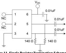
Figure 11. Single Resistor Termination Scheme
