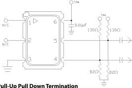
Figure 12. Pull-Up Pull Down Termination
