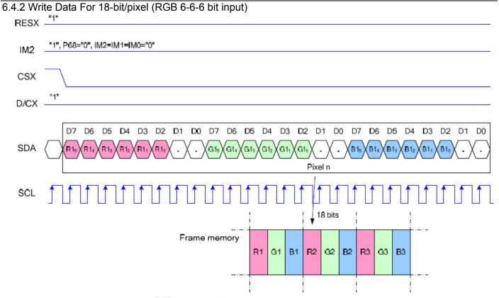
Figure 6.4.2 8-bit Data Bus GRAM Write/Read Data Format (18bit,262k)
