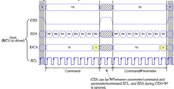
Figure 6.3.1 System Bus Interface Register Write Timing
