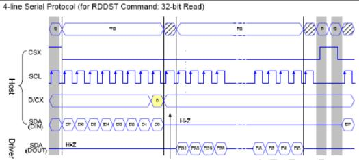
Figure 6.3.2 System Bus Interface Read Register Timing
