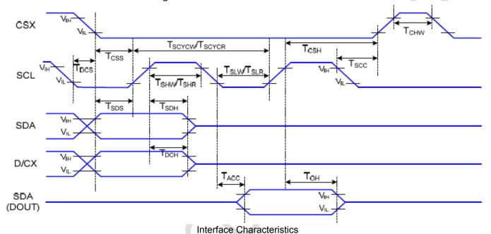
6.2 4-Wire SPI Interface Timing Parameters
