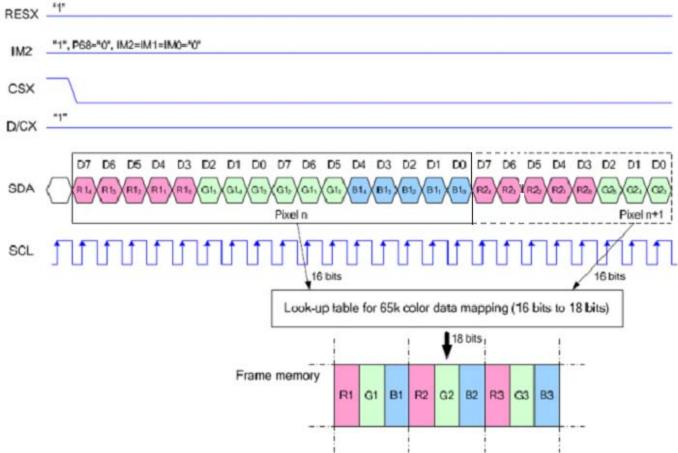
Figure 6.4.1 8-bit Data Bus GRAM Write/Read Data Format (16bit,65k)
