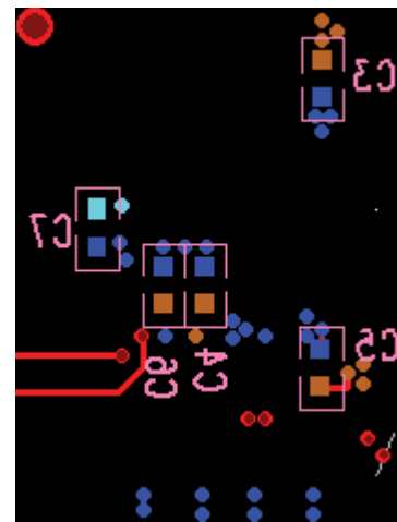
Figure 53. Bottom Layer Decoupling
