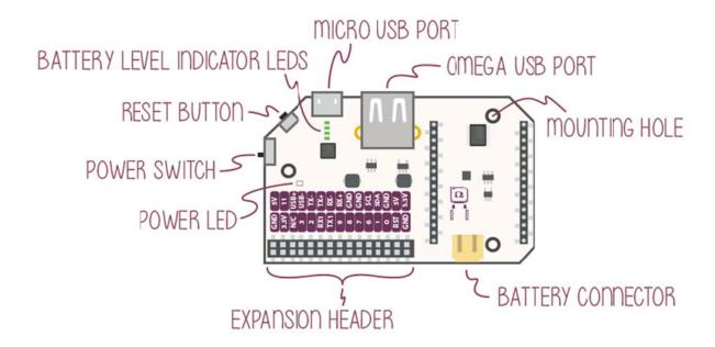
The Power Dock is flexible: it can run off just a battery or just by drawing power from the Micro USB port. Charging the battery requires having both the battery and the Micro USB plugged in. Don't worry, the Omega will still work with no interruptions while charging.
