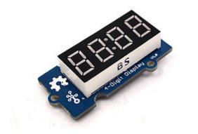
Grove - 4-Digit Display module is a 12-pin module. In this module, we utilize a TM1637 to scale down the number of controlling pins to 2. That is to say, it controls both the content and the luminance via only 2 digital pins of Arduino or Seeeduino. For projects that require alphanumeric display, this can be a nice choice.
